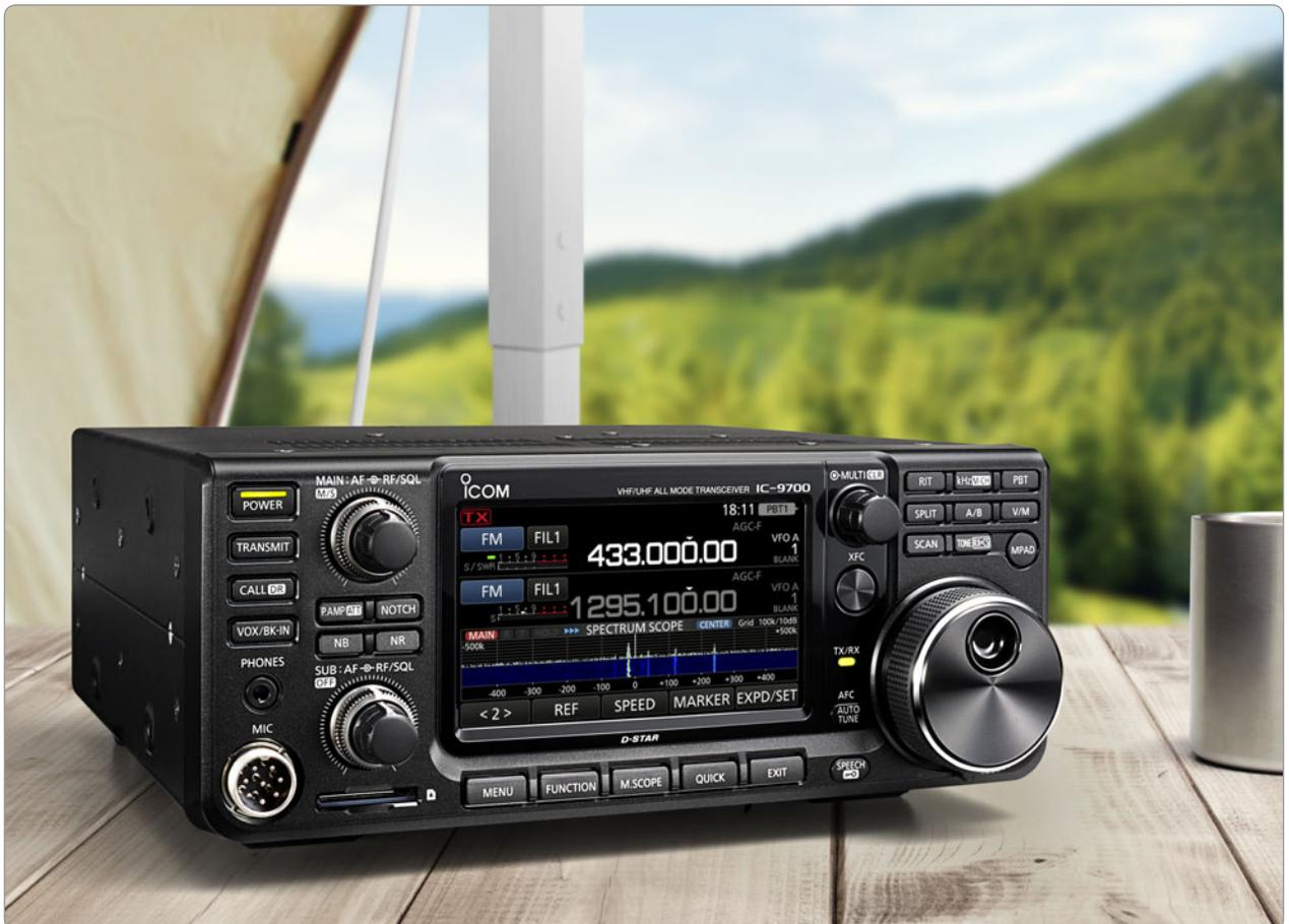
I next dialled up the local 2 m and 70 cm beacons and immediately had signals from both, right on frequency when in CW mode. I could not yet check the 23 cm beacon as I had no antenna connected.
